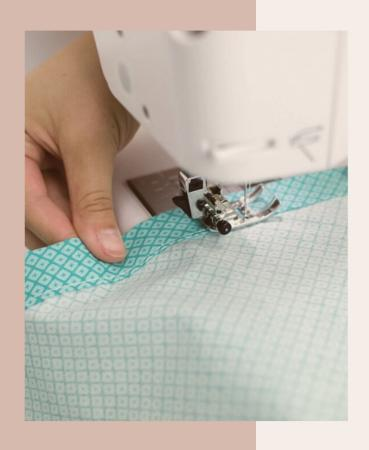
Gently guide the fabric into the sewing machine, paying careful attention to the edge. Sewing machines have lines etched into the surface beneath the needle for use as a guide. Try to guide the fabric using one of these guide lines to keep the stitch a constant distance from the edge of the hem. Don't try to go too fast. If you make a mistake, stop - you may need to remove the stitches and start over. It is far better to start over than to just keep sewing!
